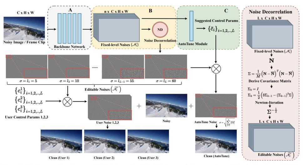
Figure 3. Pipeline overview of proposed RCD framework. A: Backbone network for generating multi-level noise maps. B: Noise Decorrelation module for editable noises. C: AutoTune module for providing reference control parameters for users.
