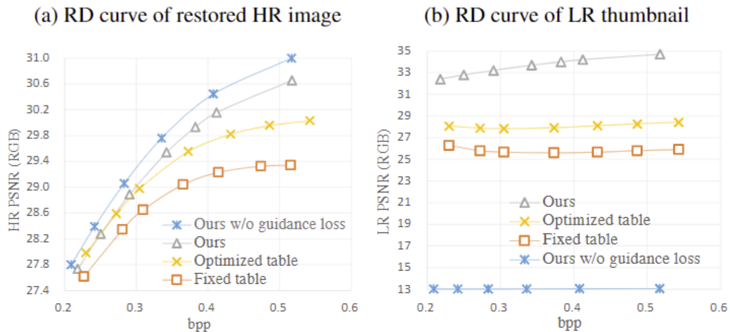
Figure 7. QPM versus image-invariant quantization. We first train our models with QPM, with a fixed JPEG table or with an optimized table, respectively. Then, we evaluate the at different target bitrate on Kodak [1] dataset. (a) the RD curve on reconstructed HR image \hat{x} and input x ; (b) the RD curve on LR thumbnail \hat{y} and the Bicubic downsampled LR y_{ref} .
