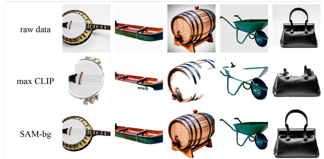
Figure 5. Examples of object mask of different annotation strategies. SAM-bg can obtain more complete and delicate masks.
